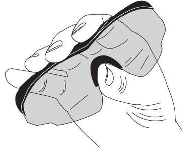
2] Position hand as pictured above and squeeze into lens until the nose piece completely seats.
