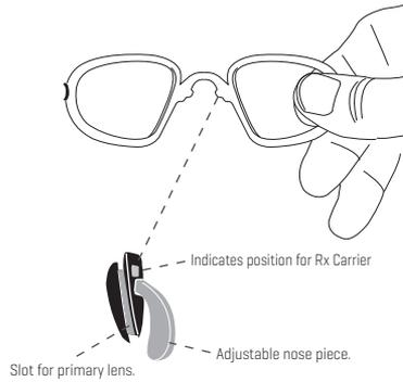
The prescription carrier is held in place by aligning the buds on the Rx carrier into the notches on the nose piece.
