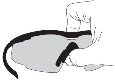
2] Align center lens slot into center catch of the frame. [see B]
