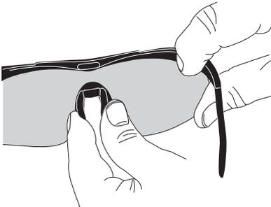
1] Ballistic spectacles protect best when the entire perimeter of the lens and frame are closest to the wearers face. For your best, most protective fit, adjust the "Take Flight" nose piece so that there is minimal gap between the lens, side of your face and under your eyes.
