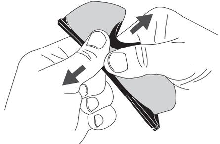
Position one hand to grasp the frame at the center of the brow bar, the other hand directly opposite at the nose piece / lens junction, as pictured. Simply pull apart.
