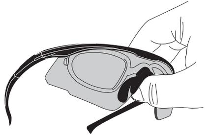
Position hand as pictured above and squeeze into lens until the nose piece completely seats.
