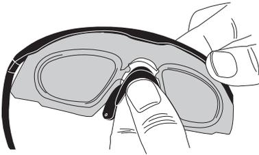
Align the groove of the nose piece,
