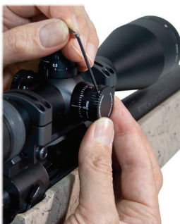
Align the windage turret cap.
