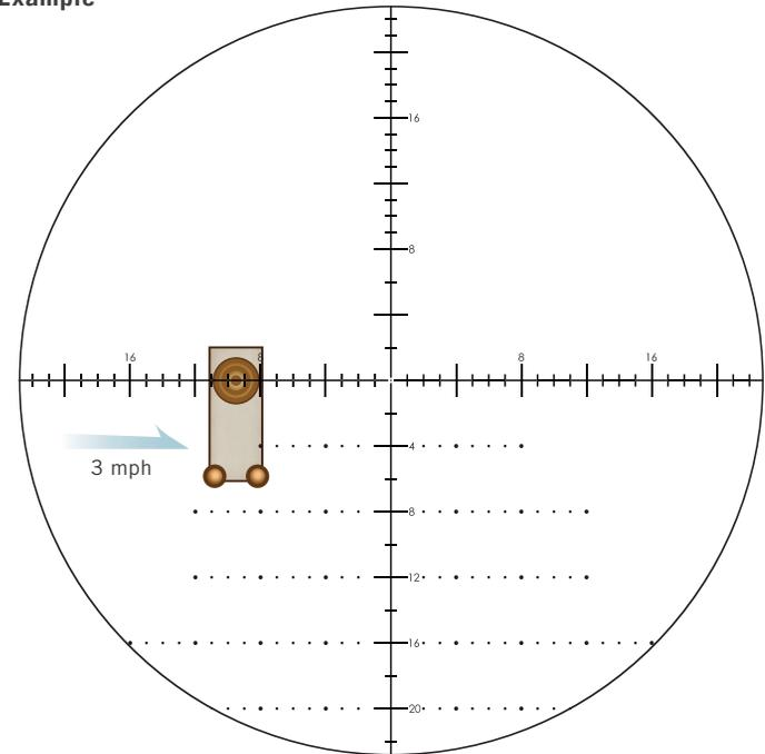
9.5 MOA reticle correction for a target moving at 3 mph at a distance of 800 yards. No wind. Elevation adjustment already dialed into riflescope.
