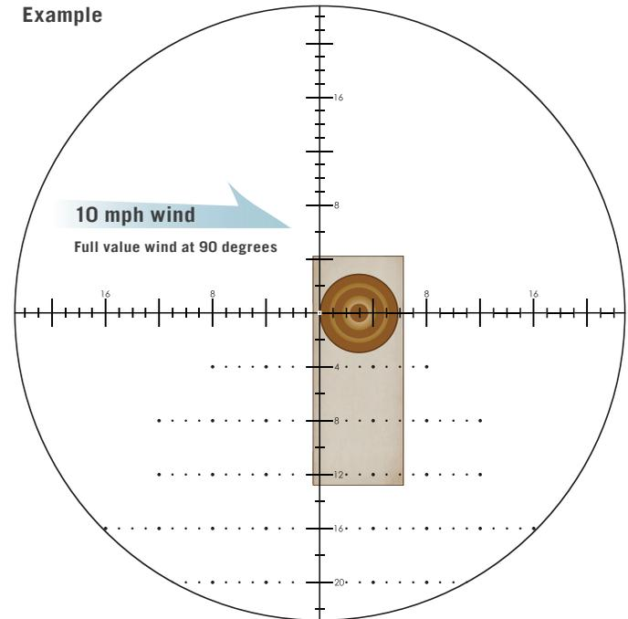
3 MOA reticle windage correction for 400 yard shot in 10 mph crosswind using center crosshair. Elevation adjustment already dialed into riflescope.
