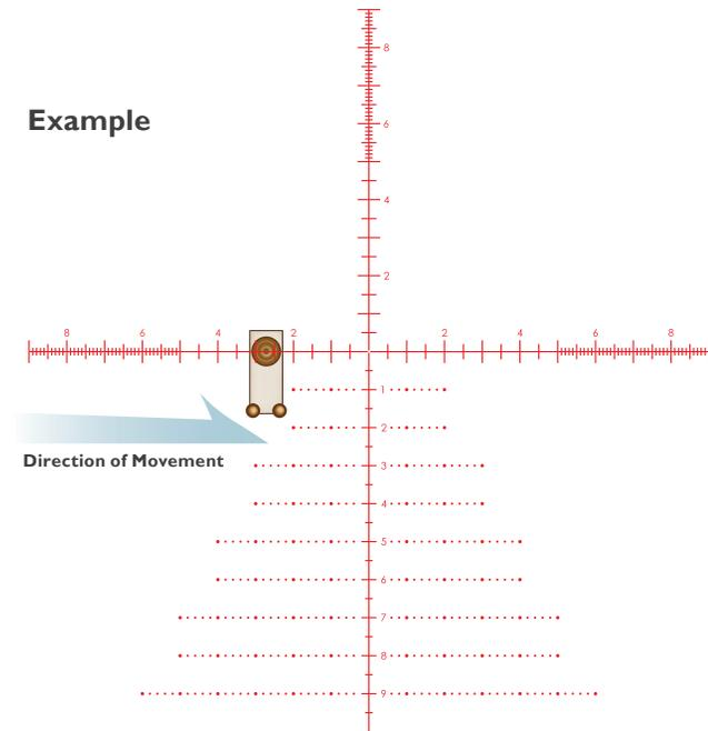
2.74 mrad correction for a target moving at 3 mph at 800 yards. No wind. Total bullet time of flight from trigger pull is 1.5 seconds during which the target travels 6.6 feet. Elevation already dialed into turret.
