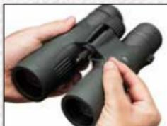
3. Using the 1.3mm Allen wrench, tighten the set screw in the threaded stud. **DO NOT OVERTIGHTEN.**
