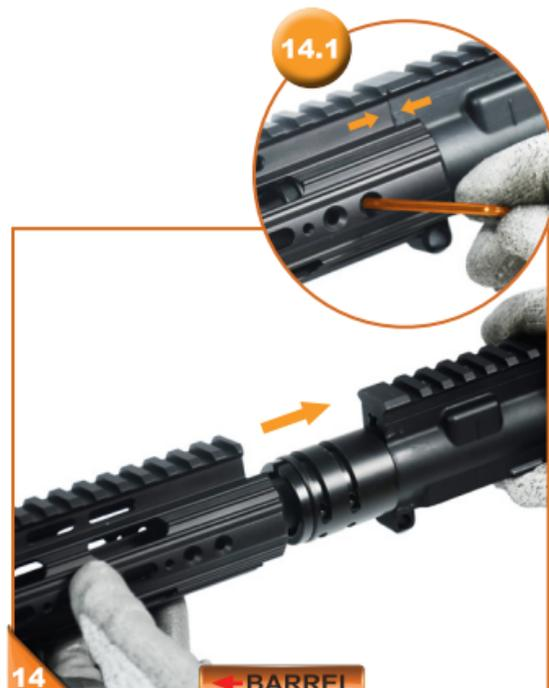
Carefully slide the handguard over the Barrel Nut/Locking Ring assembly. Make sure there is a positive connection between the top rail of the handguard and the top rail of the receiver (there should be NO gap here). If you lose the alignment of the Locking Ring, use your Allen wrench to re-align the threaded holes (14.1).
