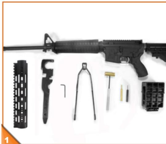
1 Prepare the rifle, the mount and necessary tools (an AR-15 combo wrench, 3mm Allen wrench, an AR-15 handguard removal tool, a hammer, a punch, an AR-15 upper receiver vise block, and a vise). Set up a comfortable working environment.
