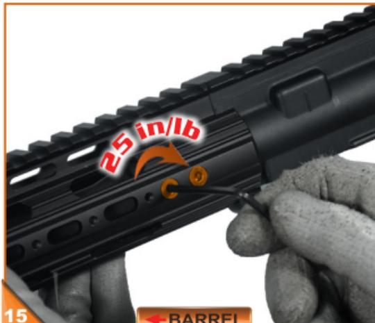
Once you achieve the proper alignment of the threaded holes on the Locking Ring to those on the handguard rail, use 6 of the Locking Screws to securely lock the handguard to the Barrel Nut/Locking Ring assembly.
