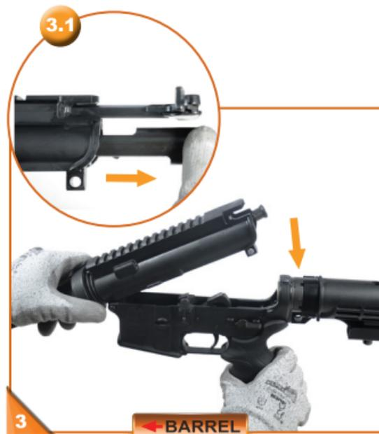
3 Remove the lower receiver with stock assembly. Take out the bolt assembly (3.1).
