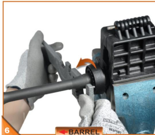
Clamp the upper receiver on a vise with an AR-15 upper receiver vise block. Loosen the barrel nut by turning it counterclockwise with an AR-15 barrel nut wrench. Take out the original barrel nut with the delta ring assembly.
