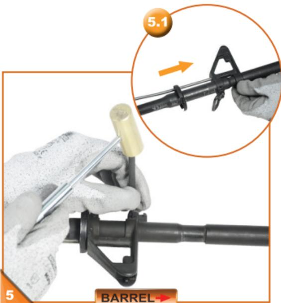
Securely place the barrel on a well padded flat surface. Punch the two pins at the bottom of the front sight out with a hammer and a punch. Remove the front sight with the gas tube, and take out the front cap (5.1)
