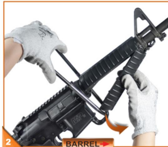
2 Remove the original plastic handguard with a handguard removal tool.
