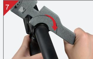
Securely tighten the Castle Nut with an AR15 armorer's wrench. Do not over tighten.
