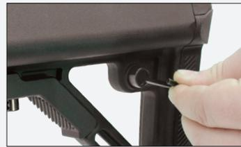
The Reversible QD Sling Swivel Housing can be installed on either the right or left side of the stock to accommodate left or right handed shooters. Use a 1/8" Allen wrench and a 5/16" socket for installation.
