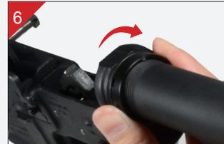
With the Tear-Drop Ring held in place, hand tighten the Castle Nut by rotating clockwise until the Tear-Drop Ring is flush against the lower receiver.
