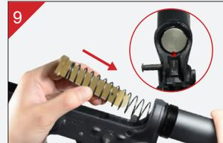
Install the Recoil Spring and Recoil Buffer into the Extension Tube until the Recoil Buffer clicks into place against the buffer detent.
