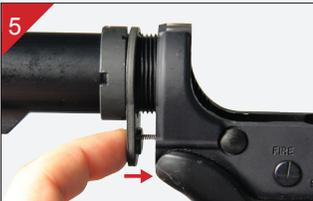
Press the Tear-Drop Ring into the receiver while making sure the take down pin detent spring goes straight back into the recess of the lower receiver.
