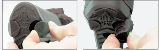
Remove either of the rubber end caps by firmly pulling it away from the stock and pulling outward until it clears the battery channel. Once batteries are inserted into the chamber, plug the rubber end cap back in securely.
