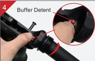
With the Tear-Drop Ring and Castle Nut in place on the Extension Tube, Install the Extension Tube into your lower receiver by pressing the buffer detent down and threading the Extension Tube until the tube overlaps the shoulder of the buffer detent. Make sure the Extension Tube is positioned correctly with the 6 position holes pointing downward.
