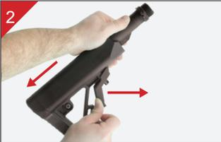
Remove the Stock from the Extension Tube by lifting up on the Adjustment Latch while simultaneously sliding the Stock off the tube. Remove the Castle Nut and Tear-Drop Ring from the tube.
