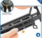
Place the Bottom Rail Cover underneath the barrel, making sure the non-tapered end of the cover is facing towards the muzzle. Seat the tapered rear of the Bottom Rail Cover so that it will slip underneath the Delta Ring by first pushing back on the Delta Ring with it. With the Delta Ring depressed, index the Bottom Rail Cover Spinal Cord with the corresponding Barrel Nut Groove
