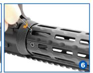
Secure the two rail covers together by using the supplied 3mm Allen Wrench to screw in the four M4 Locking Screws. There are two screw holes on each side of the handguard. Turn the Allen Wrench clockwise to tighten. Recommended torque value: 15 in-lbs.
