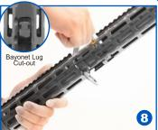
To install the Extended Bottom Rail Cover, place the cover underneath the Extended Top Rail Cover with the bayonet cutout towards the rear. Align the top and bottom rail cover screw holes. Secure the two rail covers together by using the supplied 3mm Allen Wrench to screw in the four M4 Locking Screws. There are two screw holes on each side of the extended rail cover. Turn the Allen Wrench clockwise to tighten. Recommended torque value: 15 in-15e.
