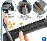
Place the Top Rail Cover over the barrel. making sure the non-tapered end of the cover is facing towards the muzzle. Seat the tapered rear of the Top Rail Cover so that it will slip underneath the Delta Ring. Do this by completely depressing the Delta Ring and indexing the Top Rail Cover Spinal Cords with the two corresponding barrel nut grooves found on the left and right side of the Gas Tube.
