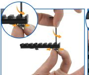
Hold the Keymod Nut in place and loosen the screw by turning it counter-clockwise with the included 3/32" Allen Wrench. Do not fully detach the Keymod Screw from the Keymod Nut.
