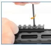
Once seated and "biased", hold the mounting base in place and retighten the T-Nuts by turning the Allen Wrench clockwise until securely tightened. Recommended torque value: 35 in-lbs.
