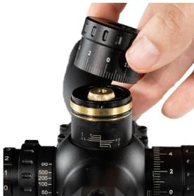
4. Locate the provided allen key and set screw. Place a dot of blue loctite on the set screw threads.
