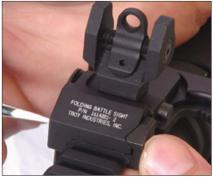
2. Apply one drop of thread locking compound to expse threads. Replace clamp and tighten screw while pushing sight forward against cross-slot.
