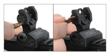
Adjustments: Can be made with a 5.56mm bullet tip (left) or a coin using the coin slot (right). To move bullet impact right, turn adjustment wheel to the right/clockwise. To move bullet impact left, turn adjustment wheel to the left/counter clockwise.
