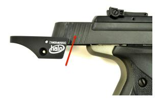
Step 3: Install and tighten the included 4-40 3/4" socket cap screws. Do not overtighten the screws. The charging handle grips tightly to the bolt. The screws should be tightened in an alternating pattern. First one and then the other then return to the first and so on until they are snug. Some blue loctite is recommended to keep them from working loose.
