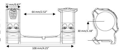
The SCT-3001D Interface Mount features two Spuhr Interface™ Top Covers, which can be installed as to position any of more than 40 different accessories in either the 12 or 3 o'clock position.
