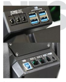
Cable management features four USB 3.0 ports, three 2.1mm power ports and three serial ports
