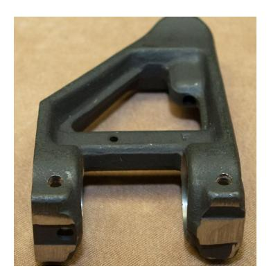
Note: Utilize care to properly align Front Sight Base to anti rotation holes on Barrel to prevent damage during re-assembly.
