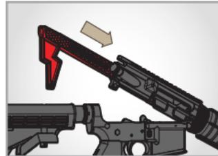
Remove bolt and insert the Smart Lock Bore Guide into the chamber
