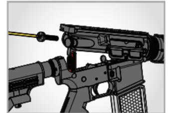
Pivot Lock provides third-hand capability to hold action of gun open while cleaning star chamber
