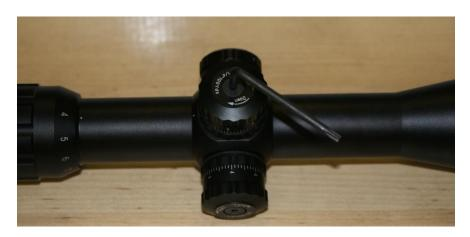
Relocate the turret to zero and replace. You might have to compress the tension ring with your other hand as you push down.
