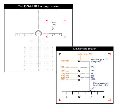
Horizontal ranging is calibrated for an 18" wide target. Simply line up the target's width with the appropriate line to determine range to target. For example, an 18" wide target that appears to be the same width as the ranging line with a "6" next to it will be 600 yards away. This method is useful when the target's height is partially obscured, as with a target in tall grass.
