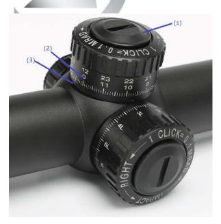
Take out the disk(1), then the turret and make the zero scale mark(2) at same level as the scale mark(3), finally screw down the disk(1).
