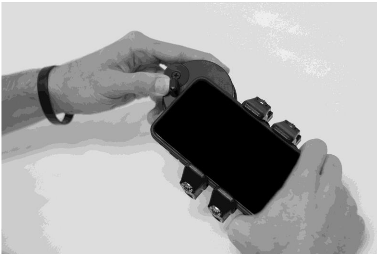
Figure 9 Rotate END STOP till it just touches phone
