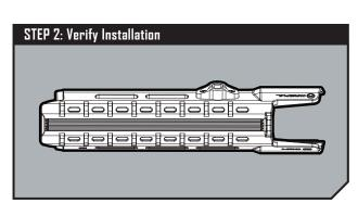
Perform final inspection including function check per US Army TM 9-1005-23&P Unit and Direct Support Maintenance Manual (3-97) to verify proper weapon function.
