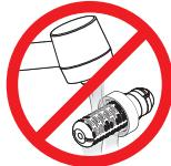
Do not rinse the EZ-Clean Membrane™ horizontally under running water – doing so may destroy the hollow fibers
