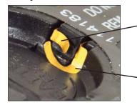
The positive contact presses against the side of the battery. When inserting the battery, make sure not to crush this contact down into the cavity.
