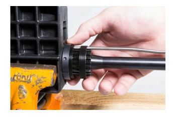
5. Thread on keymod rail on to barrel nut until aligned with rail on upper receiver.
