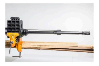
4. Screw on rail retention ring all the way on to barrel nut, do not tighten it against upper receiver.
