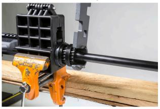
2. Check if gas tube is aligned. If not aligned, set torque wrench to 50 ft/lbs and tighten only until gas tube hole aligns, do not tighten excessively
