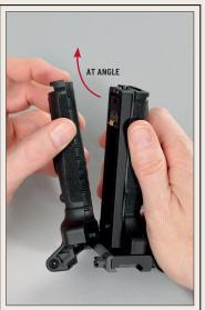
5. Slide one side off at angle to remove and release from tang.
