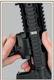
13. Bring perpendicular by rotating lugs into rail slots.
