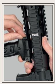
Tighten foregrip onto rail by turning nuts. Use screwdriver or nut driver to tighten. (50-55 inch/lbs.)
