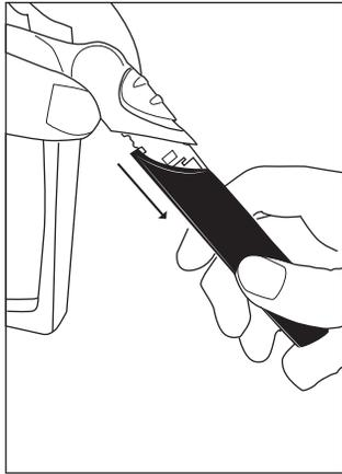
2. Insert 1 AAA battery in the correct polarity, then replace battery handle.
