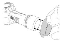
To attach reticle, line up slits in reticle with notches inside base of loupe. Press reticle into place and turn clockwise to lock.
