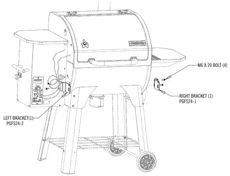
4. Install the front shelf to the brackets as shown in below.
