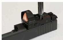
**Step 7:** Secure the FastFire 3 to the Glock MOS mounting plate using the longer screws set aside in Step 2 and two lock washers. Please contact customer service for the washers (1-888-440-0244)
