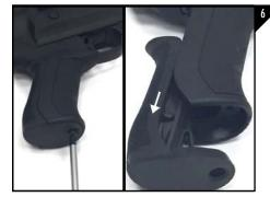
Using a Phillips Head Screw driver, remove the the 6 x 48/2 x 1/2" Phillips Head Screw from the back strap. Next, remove the back strap from the pistol grip housing as seen in Figure 6.
