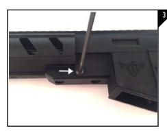
Turn the 10-22 over and using a 1/8" allen wrench remove the 10-32 Button Head Cap Screw from the left side of the forend bracket as seen in Figure 3
