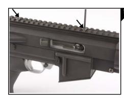
Using a 1/8" allen wrench and the (2) provided 10-32 x 5/8 Flat Head Screws tighten the the screws into the 2 holes closest to the rear of the receiver as seen in Figure 13.
