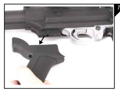
Using a 3/32" allen wrench, remove the 10-32 x 1.125" Socket Head Cap Screw from the pistol grip housing and then remove the pistol grip housing from the recevier as seen in Figure 7
