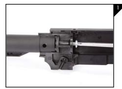
After removing the barreled action from the OEM stock, begin by placing the buffer tube so it is flush against the left side receiver cover and using a Phillips Head Screwdriver and the provided #14 x 1.5" Philllips Head Screw tighten as seen in Figure 1
