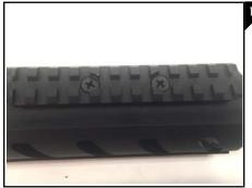
Using a 9/64 drill bit, drill a hole on each mark. Next. using the provided 10 x 5/8" Flat Phillips Head Plastite Screw and a Phillips Head Screwdriver, tighten until the screw is snug as seen in Figure 16 to complete the picatinny rail installation.
