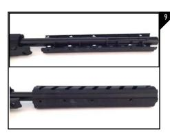
Place the barrel into the forend. Next, take the right side of the forend and snap into the left side making sure that the tabs on the right side forend line up into the pockets on the left side of the forend as seen in Figure 9.
