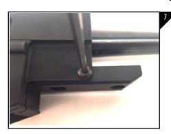
Next, using a 1/8" allen wrench and the provided (2) 10-32 x 3/8" Button Head Cap Screws tighten one of the screws into the side of the forend bracket. Flip the 10-22 over and repeat the process on the opposite side as seen in Figure 7.
