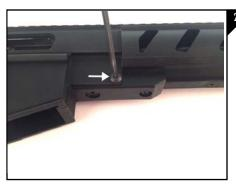
Next, using a 1/8" allen wrench remove the 10-32 Button Head Cap Screw from the right side of the forend bracket as seen in Figure 2.
