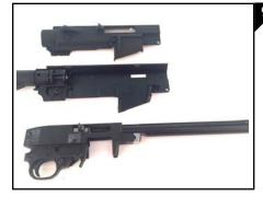
Remove the 10/22 from the left side receiver cover as seen in Figure 9. Your 10/22 is now ready to be cleaned.
