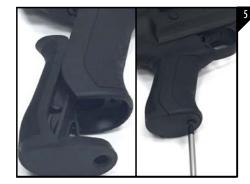
Take the back strap portion of the pistol grip and seat it into the pistol grip. Using the 6 x 48/2 x 1/2" Phillips Head Screw and the correct screw driver tighten the back strap to the pistol grip as seen in Figure 5.
