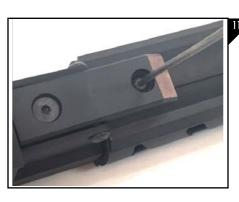
Turn the 10/22 over and using the provided 8/32 x 5/8 button head cap screw, and a 3/32 allen wrench, install into the forend bracket and tighten as seen in Figure 11.
