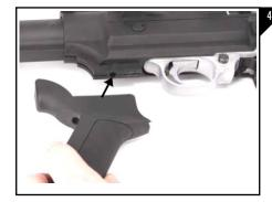
Take the front portion of the pistol grip and place it onto the stock. Using the provided 10-32 x 1.125" socket head cap screw and a 3/32 allen wrench, tighten the grip to the receiver as seen in Figure
