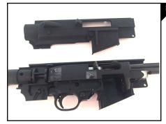
Remove the right side receiver cover from the 10/22 receiver as seen in Figure 8.
