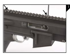
For easy cleaning of your 10/22 begin by removing the (2) 10-32 x 5/8 Flat Head Screws from the top rail closest to the rear of the receiver using a 1/8" allen wrench as seen in Figure 1.
