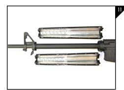
To install the bi-pod on a polymer forend begin by removing the lower handguard as seen in Figure 11.
