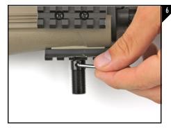
Place the 1/2 x 20 x 1-1/8 mounting column over the front sling swivel. Align the swivel stud through hole with the mounting column hole; then install and center the retaining pin as seen in Figure 6.
