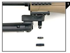
Place the mounting column washer over the mounting column as seen in Figure 9.
