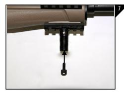
Tighten the Set Screw which you installed in step #2 and than install the new 10-32 x 5/16" threaded sling swivel stud and tighten as seen in Figure 7.
