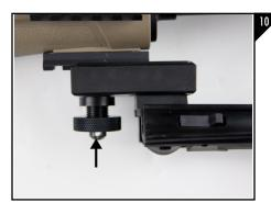
Install the 1/2 x 20 thin nut onto the column and hand tighten, plus 1/4 turn maximum as seen in Figure 10 to complete the installation. Failure to follow this procedure could result in damage to the stock. DO NOT OVERTIGHTEN
