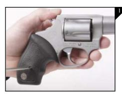
Using a flat head screwdriver remove the screw located in the side of the pistol grip as seen in Figure 1.
