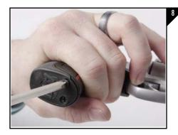
While squeezing the handle and backstrap together, install the (2) 4 x 3/8" provided phillips plastite screws and tighten into the bottom of the handle as seen in Figure 8
