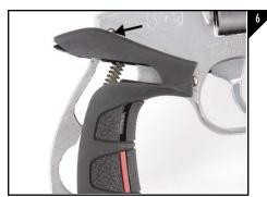
The screw seen in Figure 6 should be visible after putting the grip on or the grip has been seated to far onto the frame.
