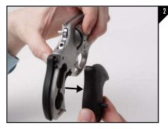
Next, remove the right side of the pistol grip by pulling out on the grip as seen in Figure 2. Repeat the same process for the left side of the grip.
