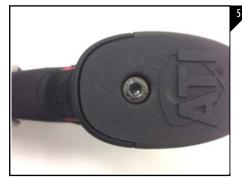
Tighten the 3mm screw until snug. The gap between the backstrap and the grip housing should be closed as seen in Figure 5. Attempt to move the grip side to side and front to back, if there is any movement tighten 1/2 turn and repeat.
