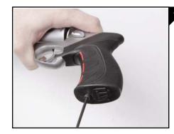
Using the 3mm screw that was removed in Figure 1, begin to tighten into the bottom of the grip using a 3mm allen wrench as seen in Figure 4.
