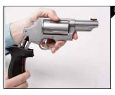
Take the X2 Scorpion Grip and slide onto the handle as seen in Figure 3. NOTE: If you disassemble the X2 grip before installation, make sure to attach the scorpion pad to the grip from the top to bottom to insure proper fitment before installing onto your Taurus.
