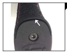
Do not overtighten the 3mm screw as it may cause the polymer to compress and create a gap as seen in Figure 6.
