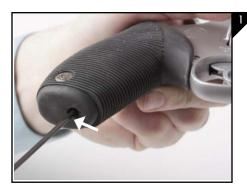
Using a 3mm Allen Wrench remove the screw from the bottom of the OEM pistol grip as seen in Figure 1.
