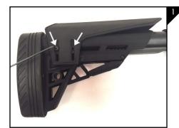
Using a 5/64 allen wrench, begin by removing the 2 6-32 x 1/4" low profile allen head screws from the cheekrest as seen in Figure 1.
