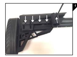
Place the shell holder onto the carrier and install the provided 10-32 x 3/8" low profile hex cap screw using a 1/8" allen wrench as seen in Figure 4. Note: You may install up to 5 shell holders.
