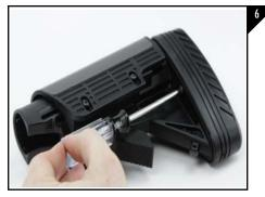
To install the Razorback Recoil Pad on the Strikeforce stock, place the buttpad on the rear of the buttstock ( do not use the plate that was included in the kit) and using a T-20 torx driver install the provided (2) 8 x 48-2 x 1/2" Plastite Torx Head Screws until snug as seen in Figure 6.
