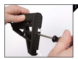
Using a T20 Torx driver remove the 2 screws from the existing recoil pad as seen in Figure 1.
