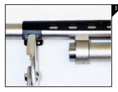
Tighten the front clamp around the barrel as seen in Figure 3.
