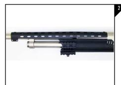
After reinstalling the barrel, slide the heatshield so that it touches the receiver, except on the Winchester which needs to be kept 1/2" from the receiver as seen in Figure 2.
