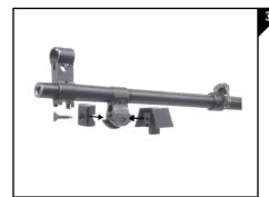
Install the bipod to the barrel by sliding the center post on the rear clamp thru the center opening of the bayonet lug. Clamp the bipod to the bayonet lug by placing the locking block over the front of the lug and use the provided #10 x 1" screw to attach to the rear clamp as seen in Figure 3.
