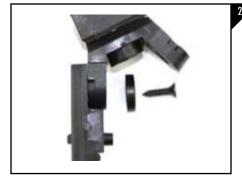
Next you will begin to install the left and right legs by inserting the post on the leg into the hole on the yoke. Using a phillips head screw driver, secure the left and right legs to the yoke with the leg mounting washers and the #10 x 3/4" sheet metal screws as seen in Figure
