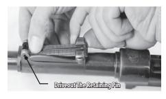
**Example (B):** Driveout retaining pin, then use small punch and tap the spring toward the front sight. Then lift out rear sight.
