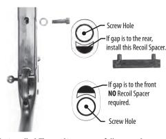
then the recoil spacer must be installed. The goal is to ensure full contact between the recoil lug and the stock. Remove the action from the stock. Insert recoil spacer, if required, into the matching holes in the stock.
