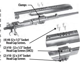
(SHCS) in the counterbored holes at the top and place the (2)  $\#10-32 \times 3/4$ " Socket Head Cap Screws in the lower side holes but do not tighten. Place the scope rail over the clamp. Install and tighten the (4)  $\#8-32 \times 1/2$ " Socket Head Cap Screws.
