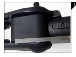
If the top folding arm is not sitting flush against the shotgun receiver, use a file or dremel tool to remove material from the notch on the top of the folding arm as seen in Figure 13. File and check often against the receiver for the proper
