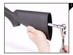
Begin by removing the existing recoil pad from your stock by using a Phillips Head Screwdriver. Next use a long Flat Head Screwdriver or the appropriate socket with extension to remove the stock bolt from the inside of the opening in the rear of the stock as seen in Figure 1.
