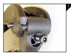
Place the appropriate bolt with supplied washer through the back of the grip and adapter (if used) as seen in Figure 7.
