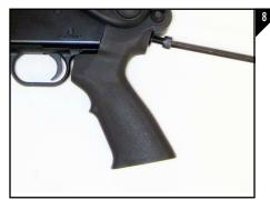
Secure the bolt to the receiver by using the proper allen wrench as seen in Figure 8.
