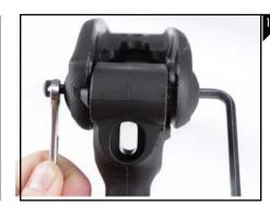
Using a 5/16 open face wrench and 3/16 allen wrench tighten until snug as seen in Figure 12. NOTE: WHEN TIGHTENING, DO NOT EXCEED 10LBS OF TORQUE.
