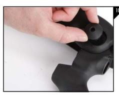
Turn the stock over and install the large TFS washer as seen in Figure 10.
