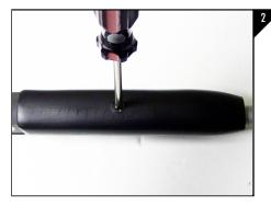
To remove the OEM forend from your H&R/ NEF shotgun, begin by unscrewing the phillips head screw from the bottom of the forend as seen in Figure 2 and then pulling downwards to seperate the forend from the barrel.
