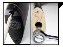
To remove the stock from your H&R/NEF, begin by removing the existing recoil pad from your shotgun by unscrewing the (2) phillips head screws in the rear of the pad. Next, using a 9/16" socket with extension, remove the bolt from the inside of the opening in the rear of the stock as seen in Figure 1.
