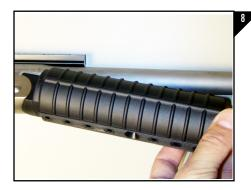
To install the Shotforce Forend, begin by aligning the rear of the forend with the front of the receiver and then pivoting the forend upwards into place as seen in Figure 8.
