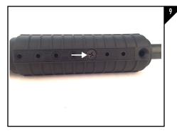
Secure the forend to the barrel by installing the provided 3/4" Phillips Head Screw and a phillips head screwdriver as seen in Figure 9.
