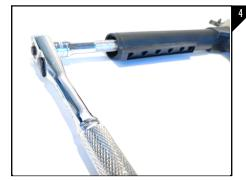
Using the provided 1 1/4" Hex head bolt and a 9/16 socket, secure the buttstock to the receiver as seen in Figure 4.
