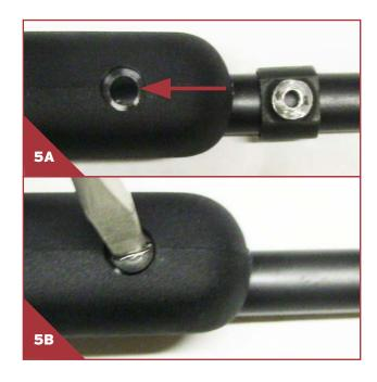
Next, align the tigger guard back into place so the trigger is properly engaged with the sear as seen in Figure 6.
