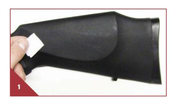
Wait 30 minutes until the alcohol is dried. Remove the backing from the adhesive pad and align the pad to the stock as seen in Figure 2.
