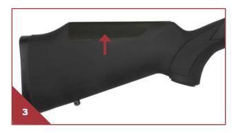
Use your thumb to remove any air bubbles in the pad and to firmly press and secure the adhesive pad onto the cheekrest as seen in Figure 4.
