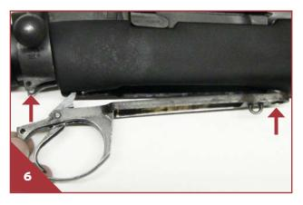
Align the original trigger guard rear screw with the trigger guard rear screw hole. Begin to thread the screw in place, but do not tighten all of the way as seen in Figur e7. NOTE: Do not fully tighten the rear screw until you have aligned and tightened the trigger guard front screw.
