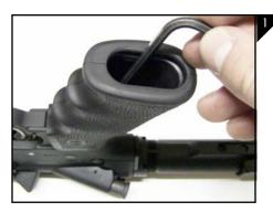
Begin by flipping the gun over and locating the bolt inside your current grip stock. Loosen the applied screw with a 3/16" standard allen wrench, and begin removing the grip as seen in Figure 1.
