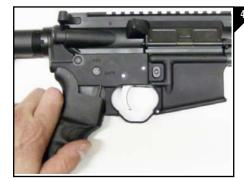
Insert the safety selector spring into the designed hole on the ATI AR-15 pistol grip. Next, slide the pistol grip into place as seen in Figure 4.
