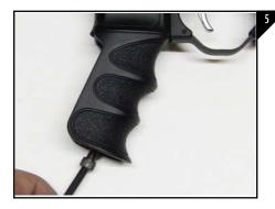
Insert the grip bolt through the bottom of the grip and tighten using a 3/16" standard allen wrench as seen in Figure 5.
