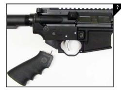
Continue to remove the grip completely. Be careful to remove the safety selector spring from the grip as seen in Figure 2. Keep both the safety selector spring and grip bolt for later installation.
