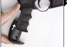
Re-install the Scorpion Recoil Pad by sliding it upward into the pistol grip as seen in Figure 6.
