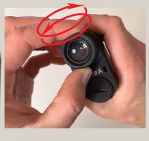
3. Adjusting the Red OLED Display Brightness: Hold the Mode Button to enter the menu setting, Press the Power Button to cycle between 5 different brightness levels. Press the Mode Button to select.
