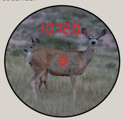
The angle-corrected Horizontal Distance (H) value is displayed at the bottom of the display for up to 8 seconds or until you take a new measurement.
