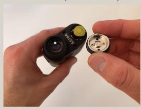
2. Turn on unit and Adjust Eyepiece
