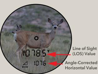
◆ The **Angle** value will flash for 2 seconds on the bottom line following the horizontal distance.
