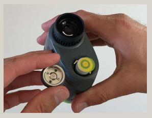
2. Turn on unit and Adjust the Eyepiece Diopter Focus: Press the Power (Range) Button to turn on the rangefinder LCD display.
